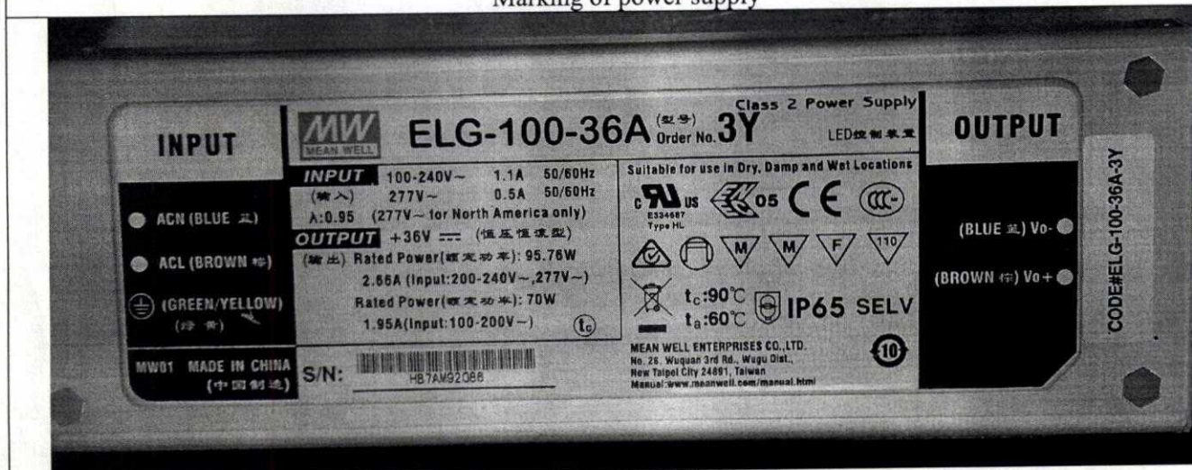
Marking of power supply
